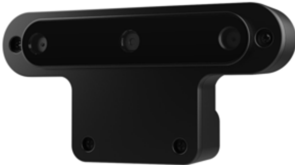
Figure 3.4 Stereo/RGB cameras from OpenCV AI kit
