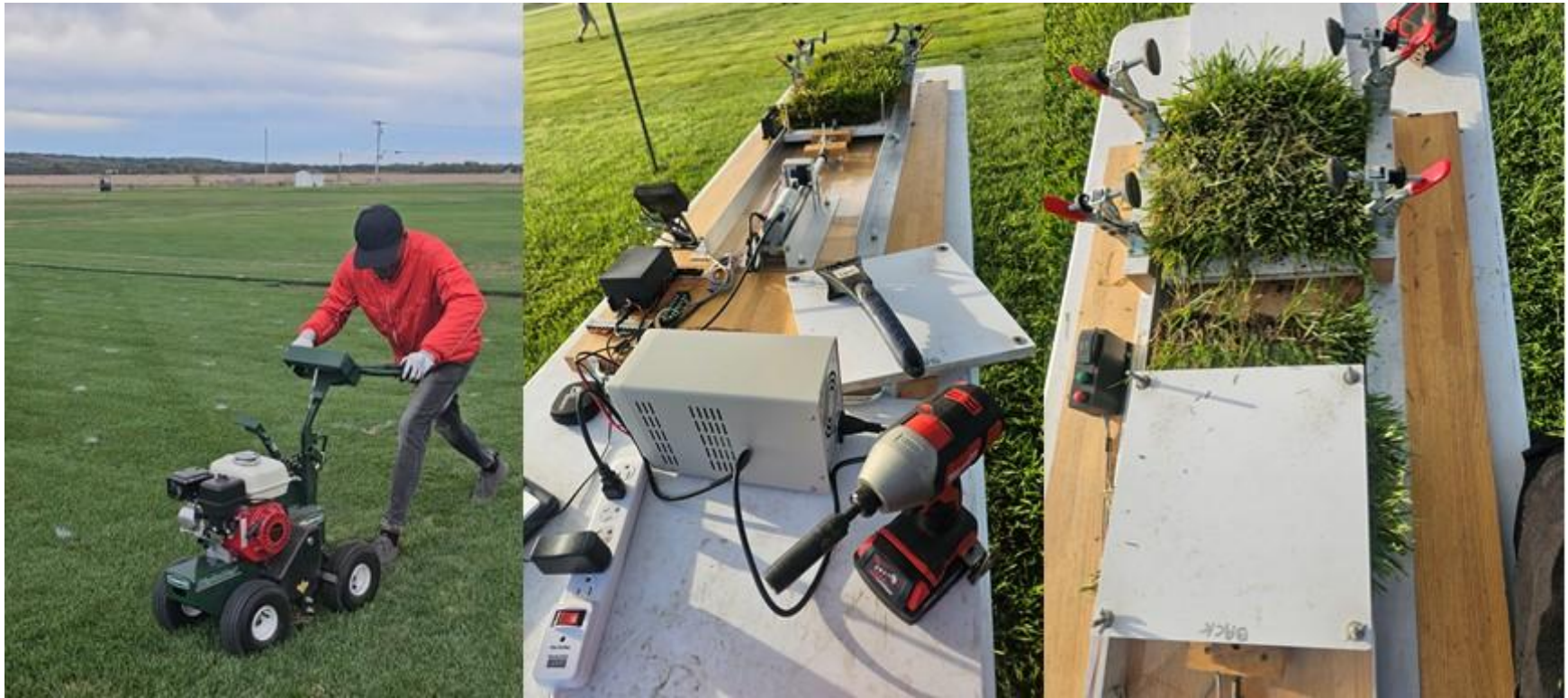
Figure 2.1. Cutting sod across plots using a Turfco KisCutter (left); Sod tensile strength device used to measure sod strength (middle); and Piece of torn sod from the sod tensile device (right) at the Rocky Ford Turfgrass Research Center, Manhattan, KS. Left photo by Ross Braun, middle and right photo by Emmanuel Nwachukwu.
