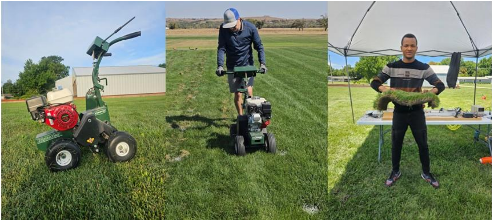
Figure 3.1. Turfco KisCutter sod cutter used to harvest sod (left), Cutting sod piece across plots (middle); Sod handling after immediately harvest (right) at the Rocky Ford Turfgrass Research Center, Manhattan, KS. Left and middle photo by Emmanuel Nwachukwu, right photo by Ross Braun.
