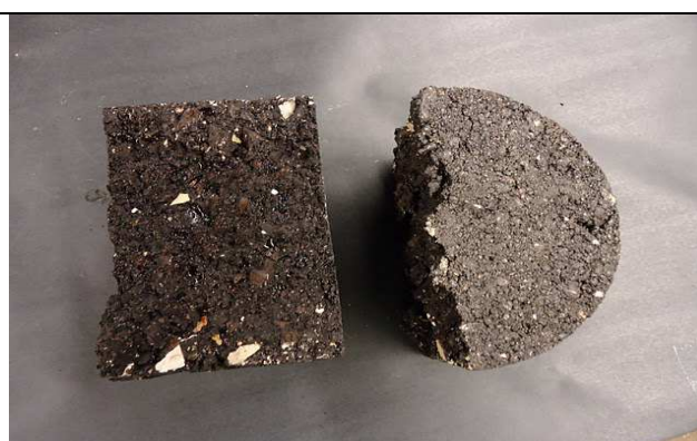
(f) Inspection of stripping on interior surface
