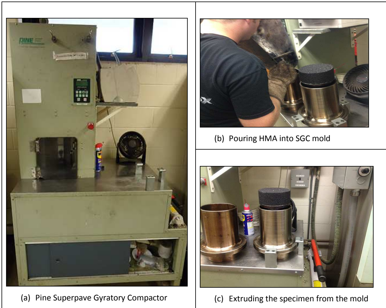
Figure 3-8. Compacting specimen using Superpave gyratory compactor
