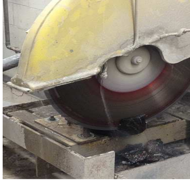
(a) Sample being cut along edge of the mold using masonry saw
