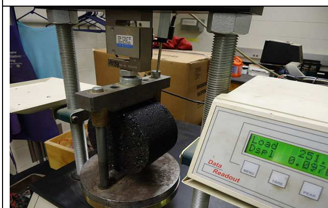
(e) Indirect tensile strength determination
