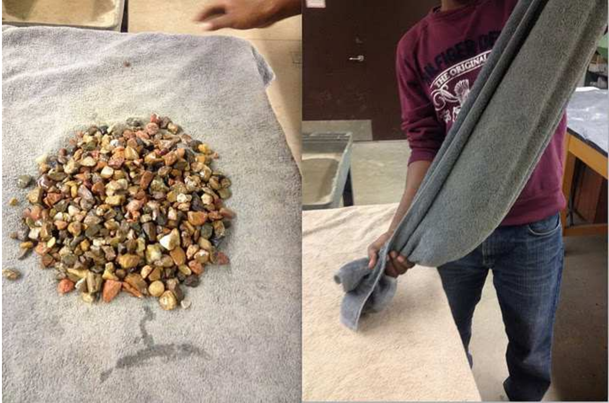
Figure 3-6. Making of saturated-surface dry condition using a dampened, absorbent towel for the coarse aggregate sample.
