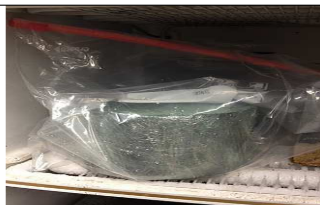
(c) Specimen freezing @ -18^{\circ}\text{C} for at least 16 hours
