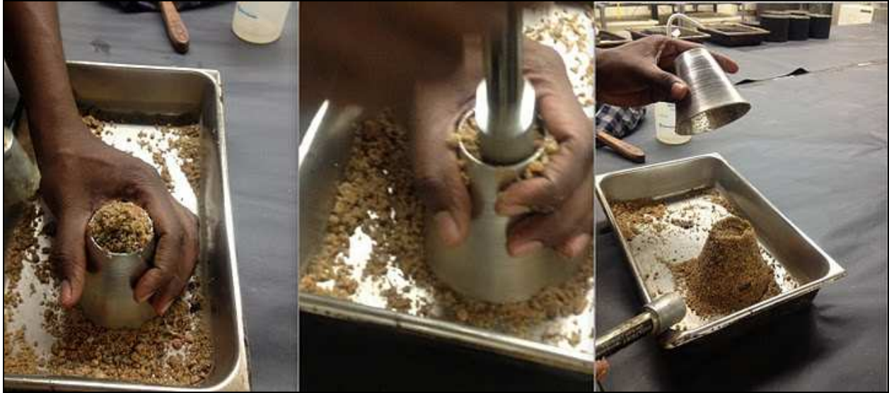
Figure 3-4. Making of saturated-surface dry condition for fine aggregate using the cone test.
