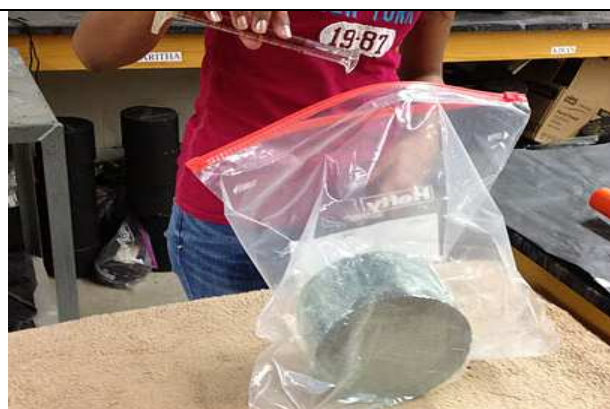
(b) Specimen wrapped with plastic film enclosed in heavy-duty, leak-proof bag with 10 ml of water
