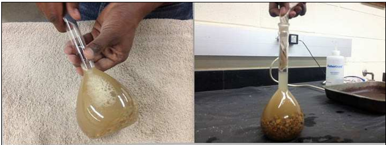
Figure 3-5. Rotation of flask in inclined position to expel all the air bubbles.
