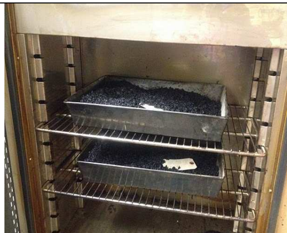
(d) Mixture kept at compaction temperature for 2 hrs (short term aging)
