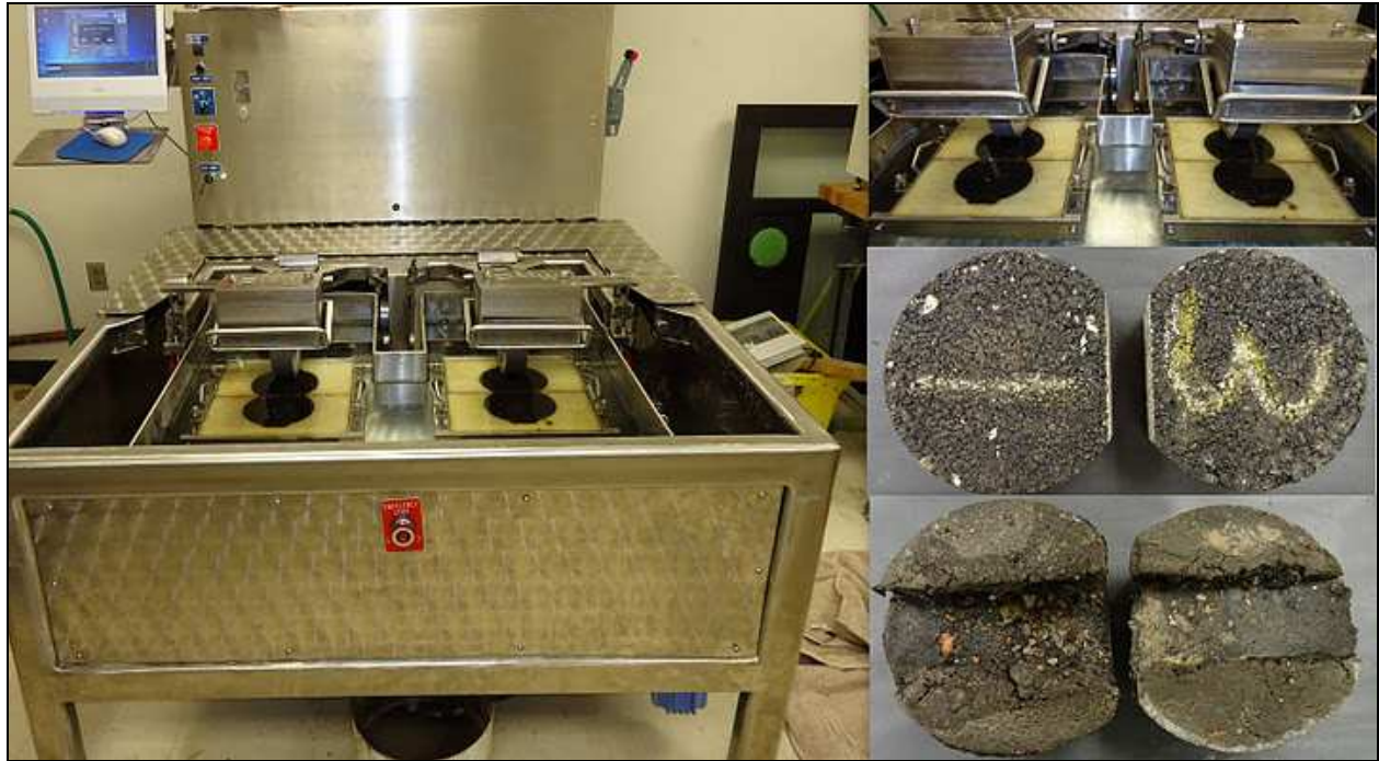
Figure 2-1. (Clockwise) Final test setup of Hamburg Wheel Tracking Device, closeup of samples under the wheel load, samples ready for testing in HWTD, and failed samples having high rut depth.
