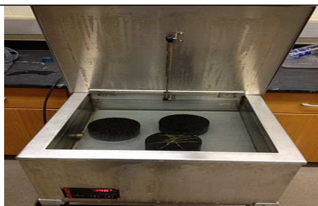
(d) Specimen in water bath at 60^{\circ}\text{C} for 24 hours
