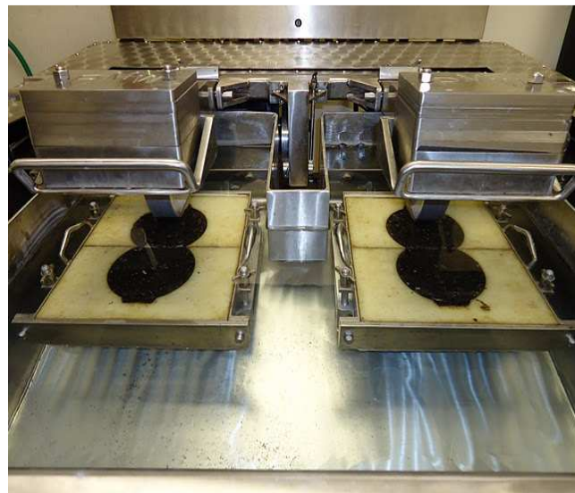
(c) Samples placed in molds and mounted in tray, ready for testing
