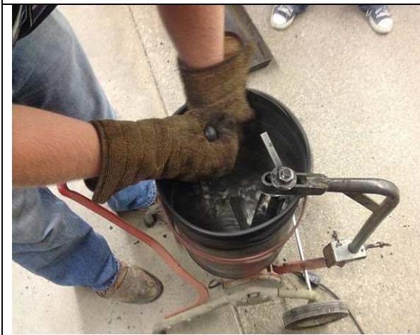
(c) Mixing of asphalt and aggregate in the mixer
