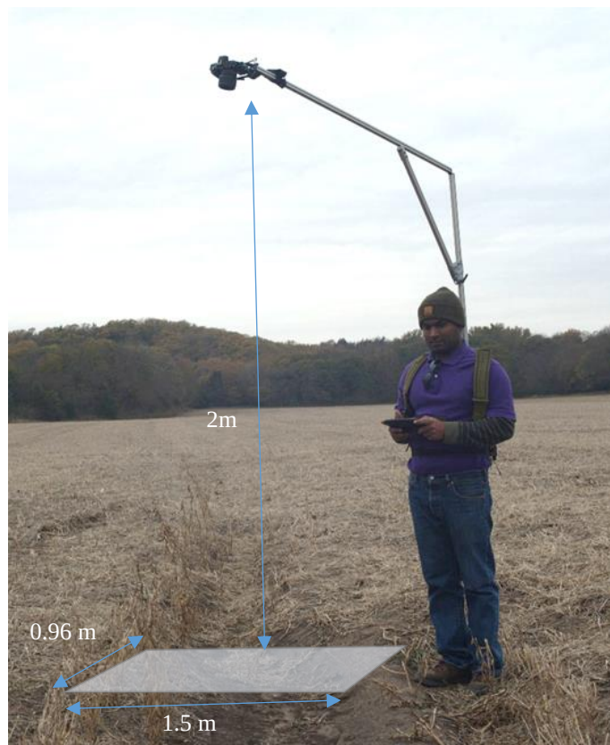
Figure 4-6: Camera setup and ground coverage area
