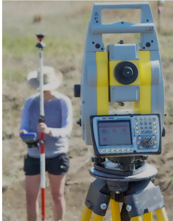
Figure 4-5: Surveying ground control points using the station survey
