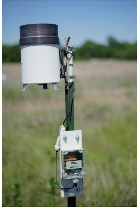
Figure 4-2: Rain gauge and data logger
